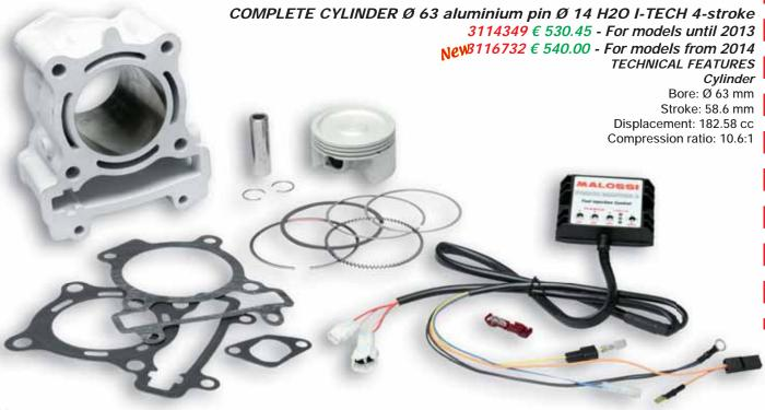
Material: primary aluminium alloy with a high content of hardened and tempered silicon, cylinder liner with silicon carbide coating in a galvanic nickel die and crossed smoothing with two diamond passages with very limited tolerances
